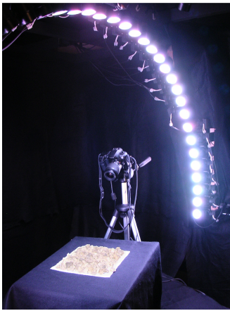
Figure 2: The setup for our data acquisition. The scene, a set of stones, and the camera are placed on a turntable. A semi-circular brace with 40 light sources is mounted over the turntable. By rotating the turntable 180 degrees in 32 steps and switching on one light source at a time, the object can be illuminated from 64 \times 20 regularly sampled directions.
