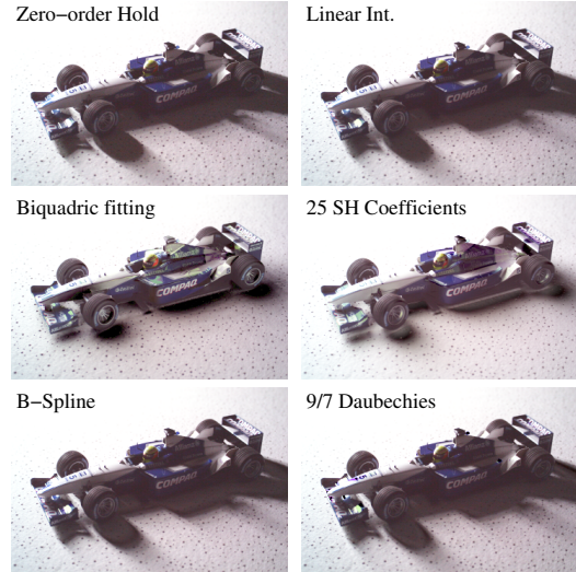
Figure 8: The miniature race car from figure 3, relit with a vertical sliver of light, using different reconstruction techniques for the reflectance functions.
