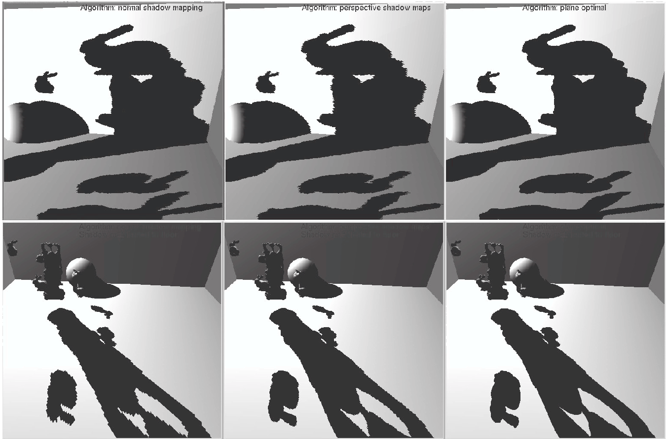
Figure 7: Left: conventional (aka normal) shadow map. Middle: Perspective shadow map. Right our (aka plane optimal) shadow map. Zoom up in viewer to observe details.
