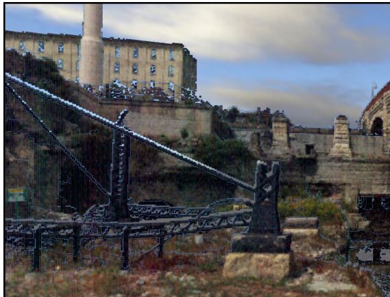
Figure 1: An attempted standard point-based rendering of scanned data. Holes and noise due to lack of data are apparent. This scene is a detail from the scene depicted in the top image of Figure 5, which is rendered in a painterly style.
