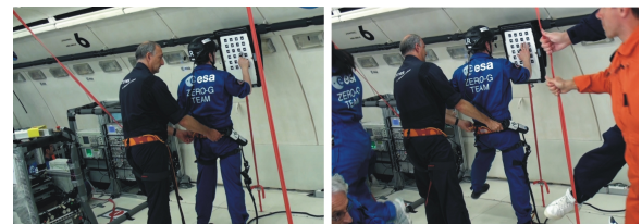
Figure 2: The PA mode under 1.8G and 0G using a surface installed at the handrail. The subject is fixed by the assistant.
