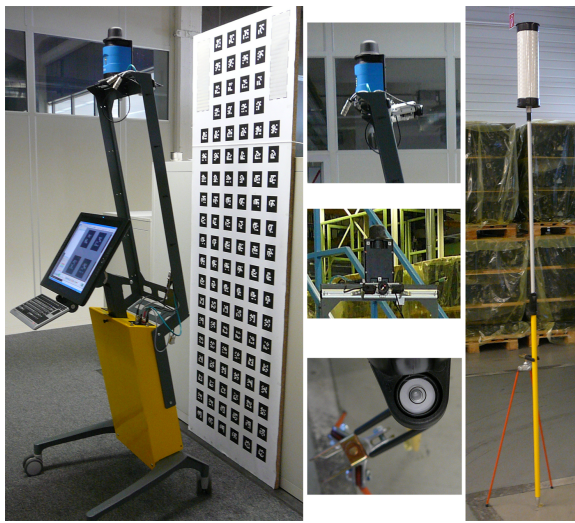
Figure 1: AR-Planar with the calibration pattern. The video camera and the servo motor (mid). To attach the cylindrical targets surveying elements are used (right). The target height is telescopically adjustable to ease the transport. A correct alignment is achieved by a water level attached to the rod (see mid bottom). The targets have a diameter of 10 cm.
