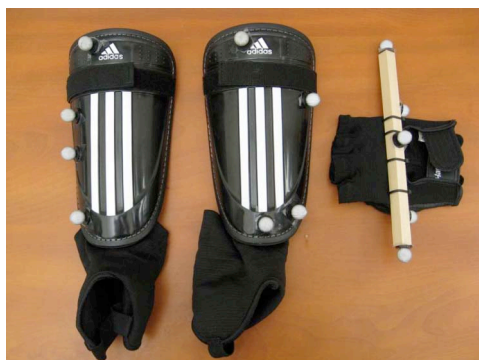
Figure 1: Shinguards and glove used for tracking.
