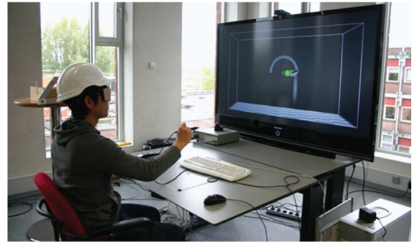
Figure 3: the experimental apparatus: a head tracked stereo display and a 6DOF input stylus.
