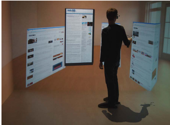
Figure 3: 2D windows are embedded into a 3D scene using a CAVE environment. The container geometry can be arranged freely in the 3D space.
