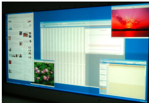
Figure 2: Our tiled display with 3 \times 2 projectors has about 4000 \times 2000 pixels. The rendering is done on 3 PCs which are controlled by a master. Each render slave is connected to two projectors.
