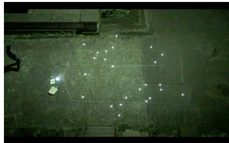
Figure 15: Large-scale display prototype one in operation; the dimensions of the prototype are 5\text{m} \times 6\text{m} and it concludes 27 LEDs. The picture is taken around 10 (m) away from the display.
