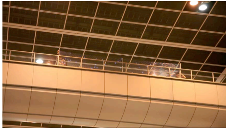
Figure 16: Large-scale display prototype two in operation; the dimensions of the prototype are 1\text{m} \times 6\text{m} and it includes 61 LEDs. The picture is taken around 15 (m) away from the display.
