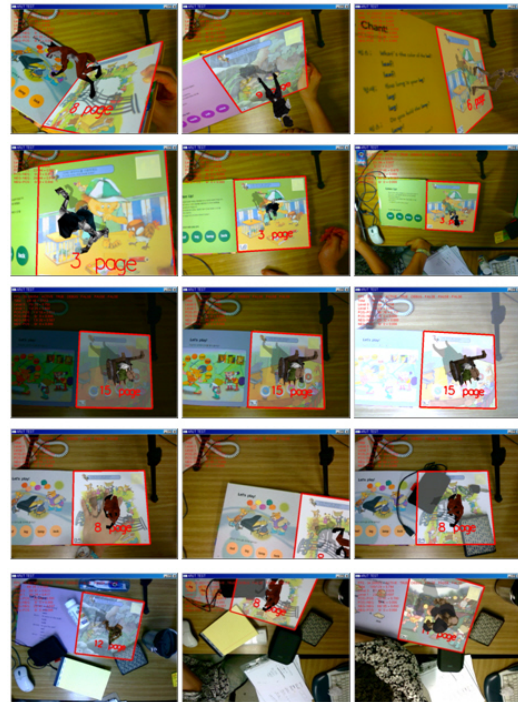
Figure 4: Tracking in situations with dramatic viewpoint variation, scale variations, illumination variations, partial occlusions, and complicated environments
