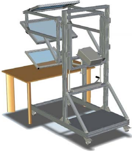
Figure 2: With its compact and mobile construction the Spinnstube® can be attached to a desk. The augmented area is created on top of a table.
