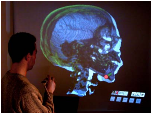
Figure 3: The "head" data-set with threshold set to bones surface. Volume in front of the cutting-plane is displayed as green contours.
