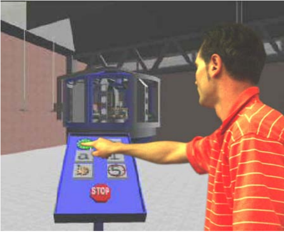
Figure 8: A user stands in front of a screen that displays rear-projected content of an interactive virtual reality application. The monoscopic projected image is linearly polarized, but can be seen by the user without any auxiliary means. The image is taken without the linear polarization filter in front of the camera lens.
