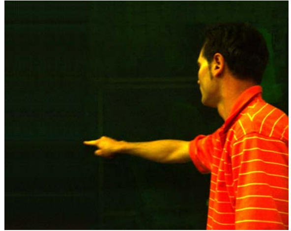
Figure 9: This image shows exactly the same scene as depicted in figure 8, but with a linear polarization filter in front of the camera lens. By properly aligning the two polarization filters in front of the projector and camera lens, the projected image can be blanked for the camera.
