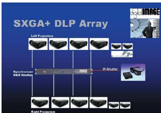
Fig. 13: Synchronized DLP Array
