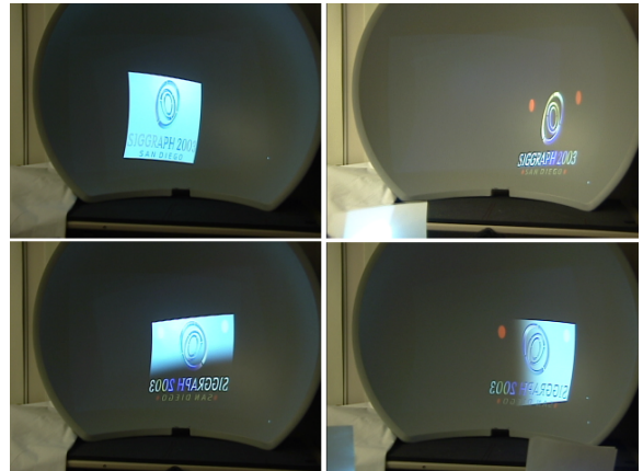
Figure 5 Four images from a sequence of accurately registered animated textured rectangles. Each of the three projectors projects a rectangle with a different texture. Projector P1 projects the rectangle textured with the “original” image. P2 projects the rectangle textured with the inverse of the original image. Similar for P3 but the inverse is augmented with red circles. The top left image shows the result with P3 entirely obscured. The top right image shows the result with P1 entirely obscured. The two bottom row images show results with P1 partially obscured.
