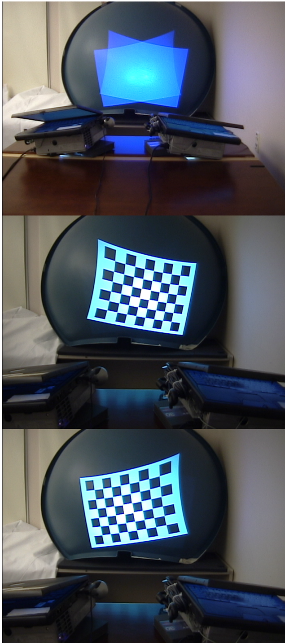
Figure 6 Two overlapping projectors on the convex, i.e. rear, side of the VisionStation dome surface.
