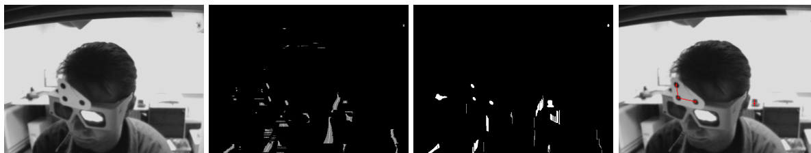
Figure 4: Algorithmic steps. From left to right: the input image, the light-dark-light regions found by the edge detector, the result of the flood fill, and the ellipses found in the original image (indicated with red crosses).
