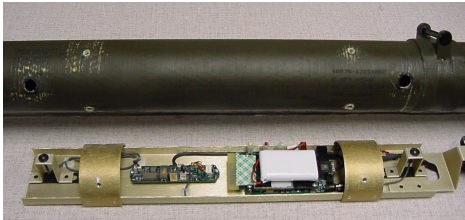
Figure 17: Tracked wireless Stinger missile weapon simulator using I 2 C interface
