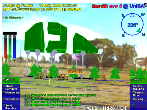
Figure 12 - AR view of constructed final model, including prefabricated street furniture items
