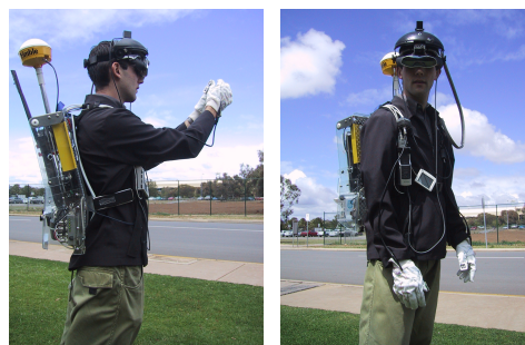
Figure 14 - The Tinmith Endeavour backpack, jointly developed by the authors at the Wearable Computer Lab of the University of South Australia with the Defence Science Technology Organisation - Salisbury
