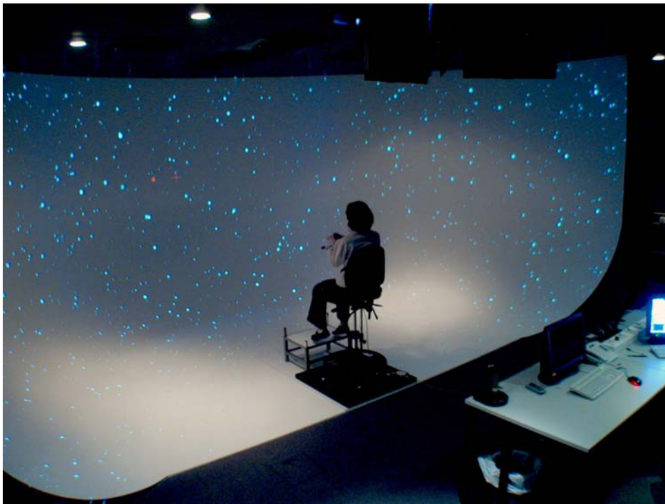
Figure 1: Panoramic screen, 230x125 degrees of field of view.
