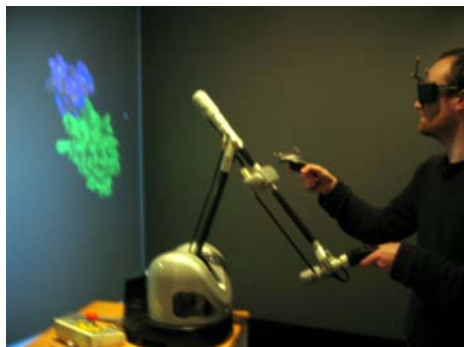
Figure 2: Bimanual direct manipulation of proteins using a 6 DOF haptic device, a tracked 3D mouse and active visual stereoscopy.
