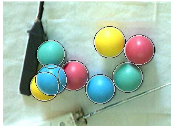
Figure 4: Performance analysis: The image used for performance analysis of the proposed algorithm. It takes 11 ms to estimate all 3D positions of these 8 color balls.
