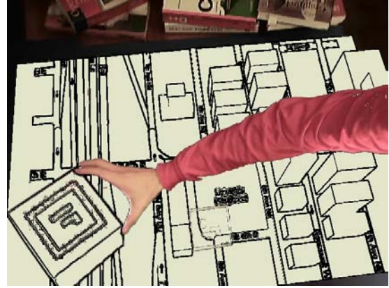
Figure 6: Selectively stylized view of the tangible interaction setup. Both virtual and real objects in the interaction zone appear in a technical illustration style. (The physical prop is visible in the lower left corner.) The real background and the user's arm and hand, however, are shown without modifications. Note that the user's arm also correctly occludes the virtual building models.
