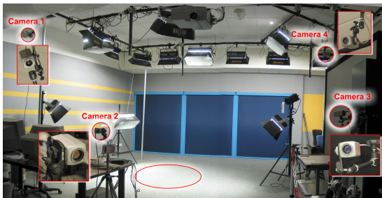
Figure 2: Experimental setup. Cameras and actor capture region are surrounded by red circles.
