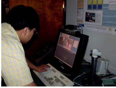
Figure 5: Prototype tele-immersive system composed of two synchronized camera, a side-by-side multiplexer, a H323 hardware codex, and an autostereo display from DTI.
