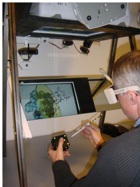
Figure 2: Two-handed interaction in a near-field virtual environment. In this example a pen and cube equipped are used to explore a molecule. A 7x7x7 cm wooden cube device with 30 circular markers arranged in 6 patterns of 5 coplanar markers, and a pen device of 4 collinear markers. Markers have a diameter of 1/2 cm.
