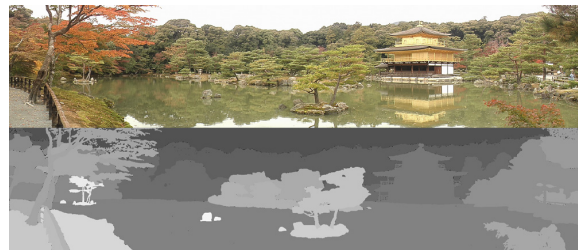
Figure 3: Generated panoramic image and corresponding disparity map (The Garden of Rokuon-ji Temple).
