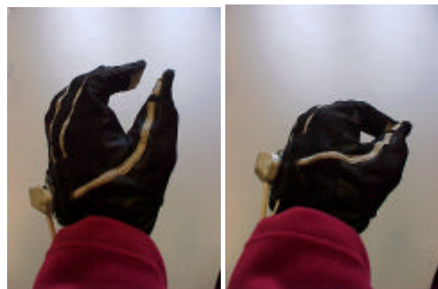
Figure 2 The "Heisenberg" effect of making a selection induces errors in the orientation of the tracker device.
