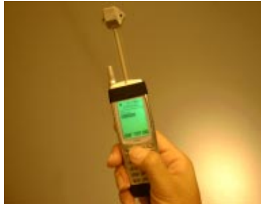
Fig. 8. Cellular Phone Interface with Pointing Function
