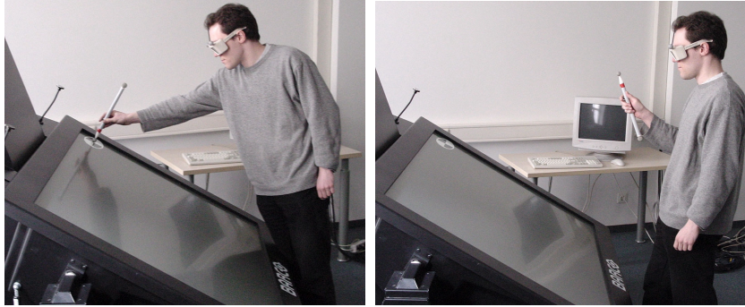
Fig. 5: Calibrating the Virtual Table: projection plan calibration (left), eye position calibration (right). For illustration purposes, the displayed marker has been enhanced.
