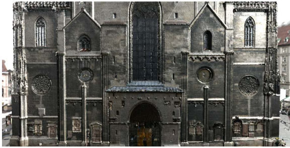
Figure 8: A huge laser scan of a cathedral ( \sim 500M points) rendered by an out-of-core point renderer with Auto Splats. The renderer streams an amount of \sim 10M points to the GPU each frame.
