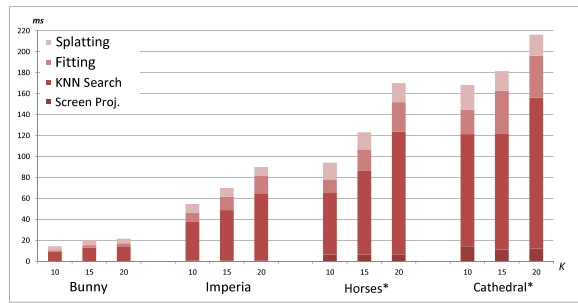
Figure 10: Performance decomposition of the computation pipeline for our test scenes for different neighborhood sizes K and 99.9% convergence. The main part of the frame time is drawn by the KNN search. The actual time for plane fitting lies in the magnitude of the final splatting stage. The horses and the cathedral scene were drawn using grid culling.
