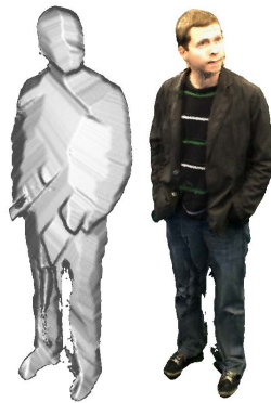
Figure 1: IBVH rendering of a person in our system. Left: phong-shaded depth map, right: same depth map rendered with view-dependent texture mapping.
