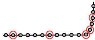
Figure 2: The encircled frames are selected for the first pass, chosen by giving equal weight to both change in direction and position of the camera.
