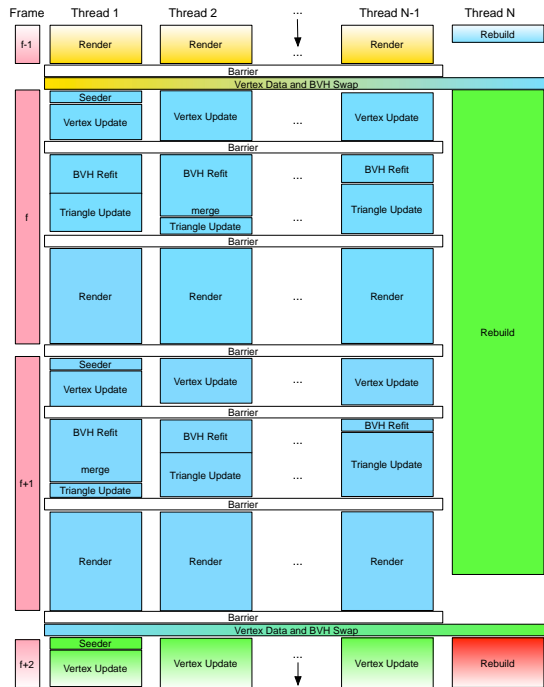
Figure 1: Given a highly parallel architecture with N cores, N - 1 of the cores work on parallel rendering and BVH refitting of the most recently finished BVH, while the N^{\text{th}} core works asynchronously and builds new BVHs as fast as possible, potentially over multiple frames (2 in this example). BVHs are deformed for only a few frames, and both scalability bottlenecks and pauses are avoided altogether.
