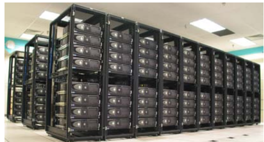
Figure 3: Visualization nodes of Sandia National Laboratories' Red RoSE cluster. The cluster has 264 visualization nodes.
