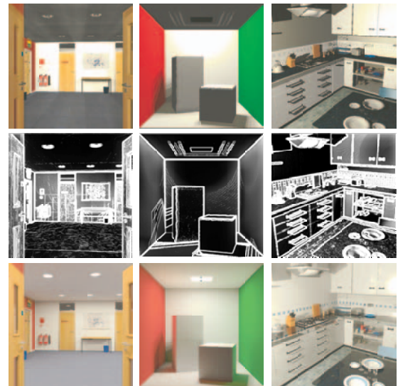
Figure 7: Test scenes. Scenes represented by image preview (top), importance map consisting of only saliency map (middle) and selectively rendered image (bottom).
