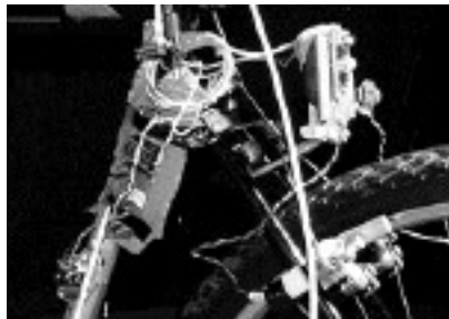
Fig. 4. The rear wheel mounting of the static bicycle shows brake sensors
