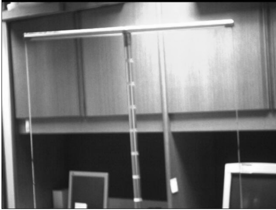
Figure 3: T shape pole for extracting the external parameters of the camera
