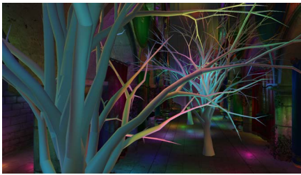
Figure 8: A view of the Crytek Sponza scene, with 10k lights randomly placed. The tree branches cause discontinuities in the depth buffer, making it more challenging for tiled deferred shading.
