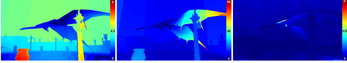
Figure 4: The required sampling frequencies are calculated using several quantities, which are shown for a frame from the ARENA scene. Left: The minimum circle of confusion radius of the primitives. Center: The minimum screen space velocity of the primitives (with constant vertex velocity approximation). Right: Span of motion directions, \hat{\theta} .
