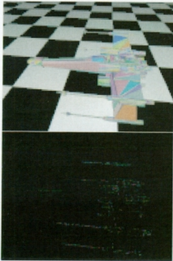
Figure 9: The x-wing fighter with 16 samples on a 16 \times 16 grid and storage for 3 fragments. The lower figure gives the per-pixel difference from a 16X sparse supersampled reference image.
