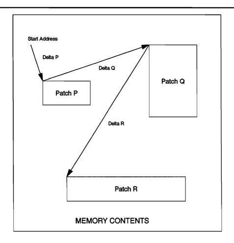
Figure 7. Variable-Patch Delta Guided Transfer
