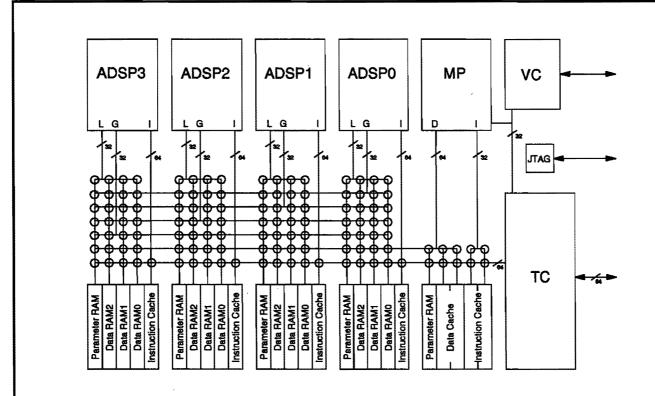
Figure 1. Block Diagram of the TMS320C80 Multimedia Video Processor (MVP)
