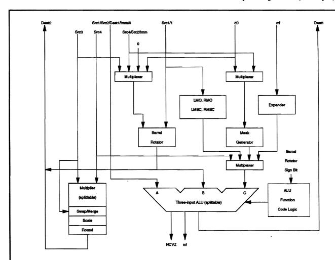
Figure 3. Diagram of the ADSP Data Unit
