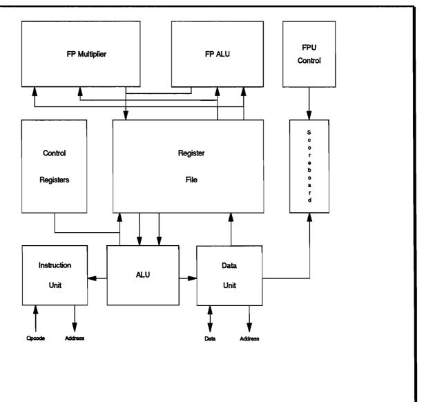
Figure 5. Block diagram of the Master Processor (MP)
