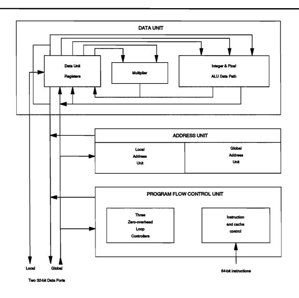
Figure 2. Block Diagram of the ADSP
