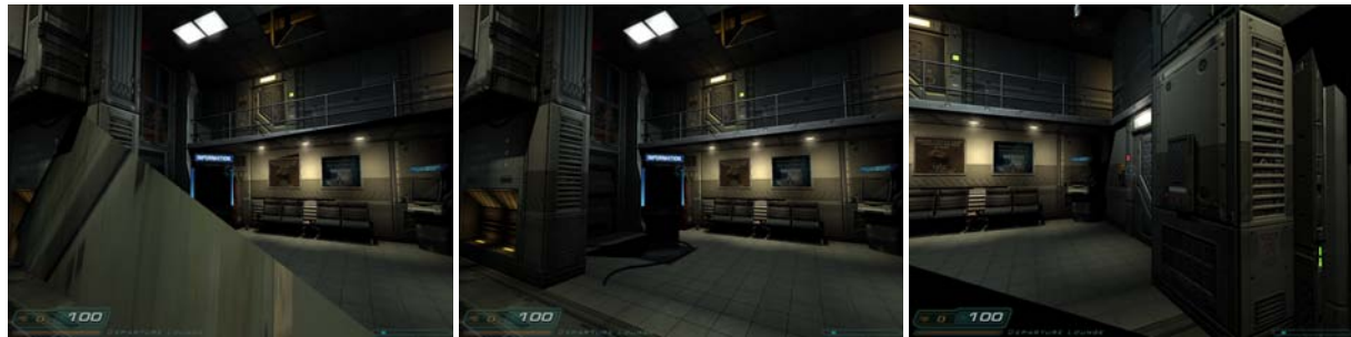
(a) A corrupted frame with 8 bits of protection (b) The same frame with 16 bits of protection. (c) Two frames before Figure 6(a). per vertex.
