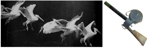
Figure 7: Multiple frames of a flying bird multiplexed into a single photograph (left). These kinds of photographs were shot with a photographic gun (right) by Etienne-Jules Marey as early as 1882.
