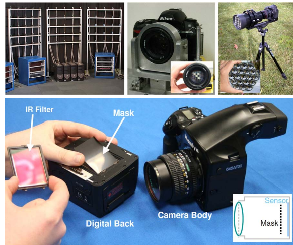
Figure 4: Light field cameras can be categorized by how a 4D light field is encoded in a set of 2D images. Methods include using multiple sensors or a single sensor with temporal, spatial, or frequency-domain multiplexing. (Top, Left) Wilburn et al. [WSLH02] describe a camera array. (Top, Middle) Liang et al. [LLW*08] achieve temporal multiplexing with a programmable aperture. (Top, Right) Georgiev et al. [GIBL08] capture spatially-multiplexed light fields using an array of lenses and prisms. (Bottom) Raskar et al. [RAWV08] capture frequency-multiplexed light fields by placing a heterodyne mask [VRA*07, VRA*08, LRAT08] close to the sensor. (Figures reproduced from [WSLH02], [LLW*08], [GIBL08], and [RAWV08].)
