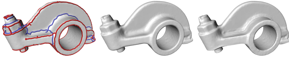
(a) Rockerarm model with some selected features in the lower part of the mesh sharpened.
