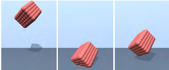
Figure 5: Sequence of a falling cuboid using [SSP07]. The cuboid deforms, but does not rotate in case of an impact.
