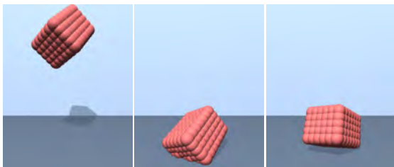
Figure 6: Sequence of a falling cuboid using the proposed corotational SPH formulation. In contrast to Fig. 5, rotations are properly handled.
