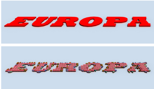
Figure 12: Comparison of the original model and the voxelized model using the real elements in Figure 11.
