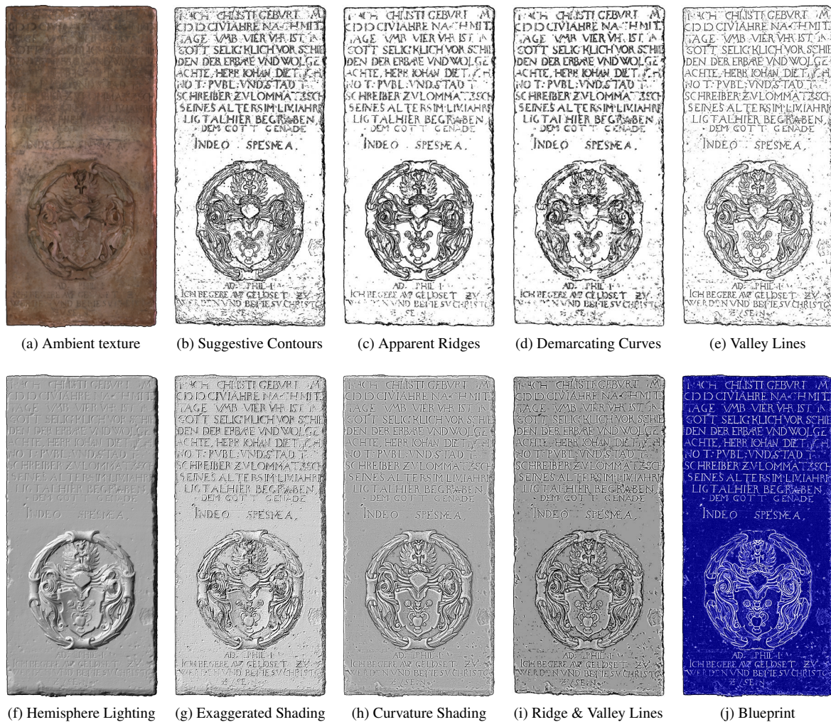
Figure 7: Several views of a 3D scanned tombstone from Lommatzsch, Eastern Saxony. Although the line drawings certainly have a better contrast than the shaded views, curvature shading has the best balance for depicting all features.
