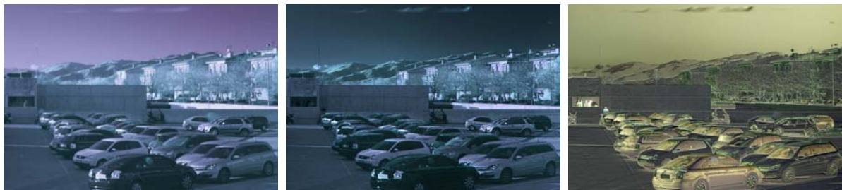
Figure 4: Near infrared image of the University Campus. The images were acquired with an infrared-converted Canon 30D camera using a Heliopan Infrared 715 NIR filter. The colors coming from the different infrared sensitivity curves of the RGB channels of the CMOS sensor. (left) Original acquired image. (middle) Image after de-polarization. Although infrared is not so rich in scattering as the bluish wavelengths, we can still remove some haze effects in NIR. Note how the details of mountains are sharper, the sky is darker due to the removed polarized intensity. (right) Degree of polarization unified in an RGB image.
