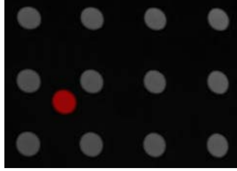
Figure 3: Example of piecewise-linear point spread function interpolation. Gray kernels correspond to images of blurred point sources, whereas the red kernel is linearly interpolated from its three nearest neighbors.
