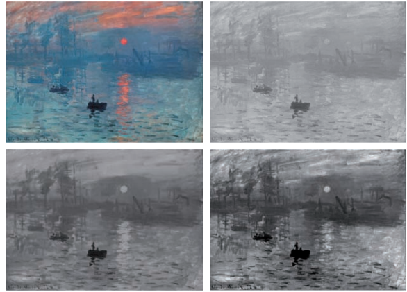
Figure 3: Comparison of our method using the CIELab formula with the CIE Y equivalent and Gooch et al. Top left: original color image, top right: CIE Y equivalent, bottom left: the result of Gooch et al., bottom right: our adaptive color to gray transformation result.
